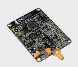
The AST family of sensor tags allows wireless measurements to be taken by sensors from remote locations. Sensors are powered by microwave energy, harvested from a dedicated RF power source and need no batteries or other consumables.
